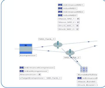
**Compressor :** mass flow rate according to the pressure of the low pressure tank
